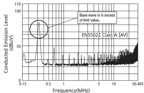
● PAN4820+PAF500Fadding external components(Capacitor: Net 3)
